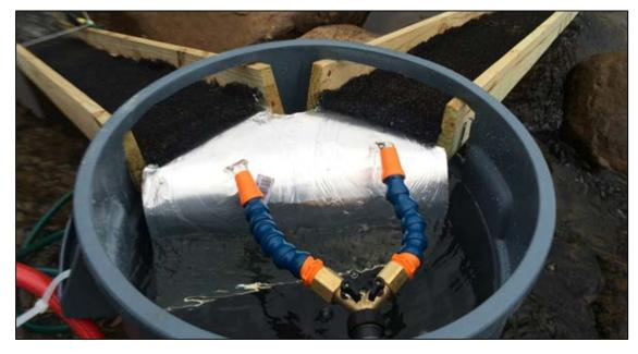
PHOTO 4 NOZZLE SETUP FOR PROVIDING FLOWS ONTO RAMPS
