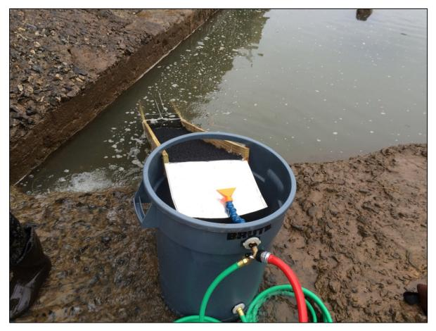
PHOTO 3 SINGLE RAMP ELVER TRAP USED IN WEST CHANNEL
