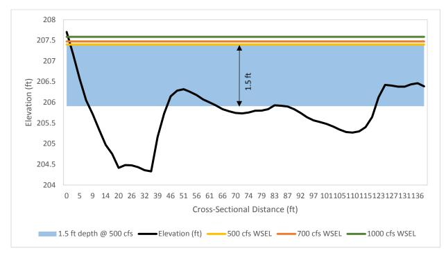
FIGURE 4-11 BED PROFILE AND WATER SURFACE ELEVATIONS AT THE RIVER LEFT PASSAGE POINT AT LEDGE 1 (UPSTREAM VIEW)
