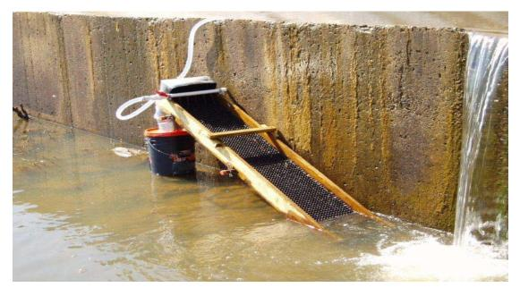
FIGURE 2. EXAMPLE OF A PORTABLE ELVER RAMP TRAP USED AT THE DOMINION PROJECT TAILRACE.
