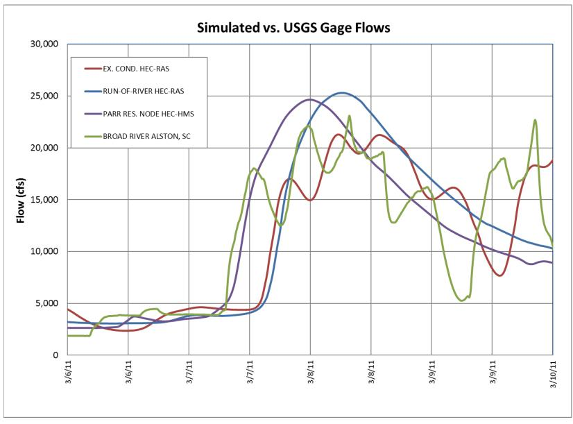
FIGURE 6 EXAMPLE OF SIMULATION OF EXISTING FLOW OPERATIONS VS. RUN-OF-RIVER ESTIMATE
