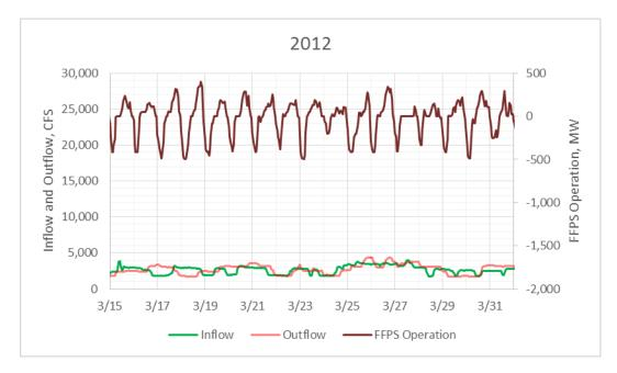
FIGURE 1GRAPH ILLUSTRATING A PERIOD OF SMALLER FLUCTUATIONS<br/>(INFLOW < PARR HYDRO HYDRAULIC CAPACITY)</th>
