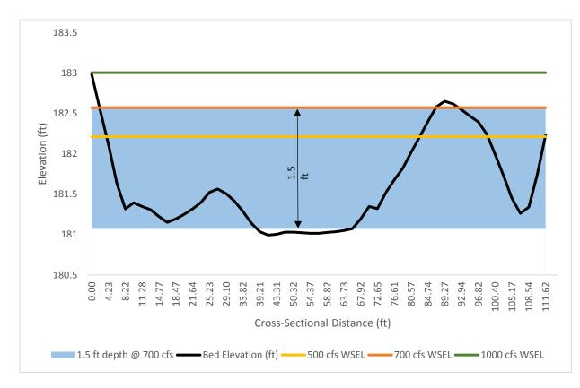
FIGURE 4-13 LEDGE 2 BED PROFILE SHOWING NAVIGATION PASSAGE AREA AT 700 CFS (UPSTREAM VIEW)
