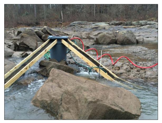
PHOTO 2 DOUBLE RAMP ELVER TRAP USED IN WEST CHANNEL
