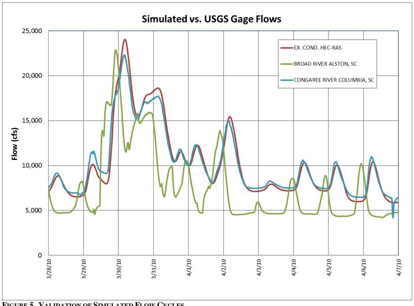
FIGURE 5 VALIDATION OF SIMULATED FLOW CYCLES
