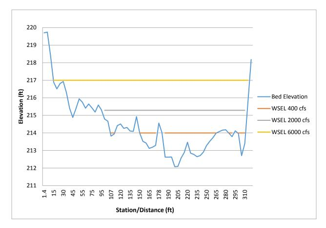
FIGURE 4-4 BED PROFILE AT STUDY SITE 4 SHOWING WATER SURFACE ELEVATION AT IFIM CALIBRATION FLOWS
